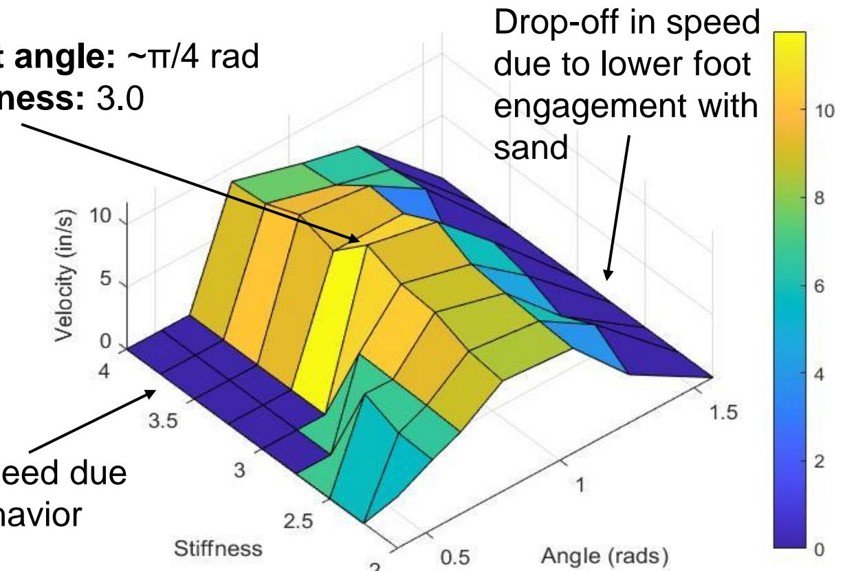
Drop-off in speed due to lower foot engagement with sand
