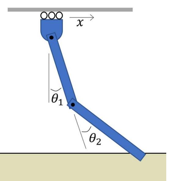
Using impedance control on a 2-DOF robotic leg, the “paddle” locomotion strategy is replicated, with the hip joint having 360 degree range of motion.
