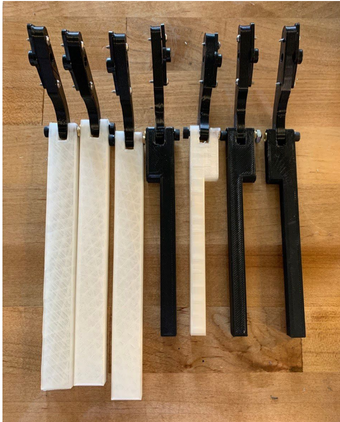
Large and Small Plungers and Connected to Corresponding Levers
